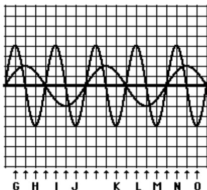
**Interference with the *Right Timing* causes Standing Waves**
