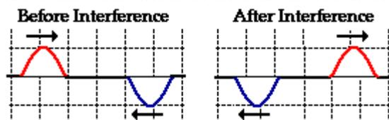
This adding or subtracting of waves that interfere with one another is called the Principle of Superposition. One application of destructive interference is in NOISE CANCELLATION HEADPHONES.
